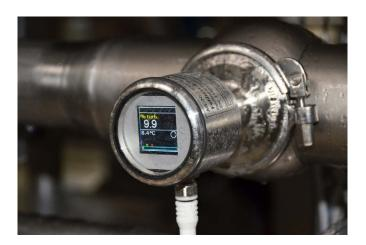
From the user's point of view, simple connection and installation also plays a relevant role in the selection of the appropriate turbidity measurement technology. Added to this are simple on-site operation and the quick and reliable ability to test the turbidity sensors used in the field and calibrate them where necessary.
